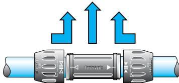
3. Remove the body and nuts of the connector. Re-tighten the nuts onto the body for future use.
