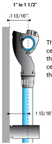
The distance from the center of the pipe to the wall is equal to the center of the bracket to the wall. (i.e. 1 13/16")
