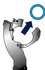
3. Position the quick assembly bracket over the hole. The bracket has a raised plug to fit into the drilled hole.
