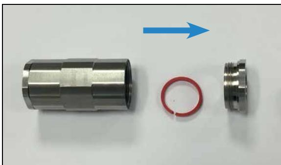
**Disassembly :** 4. Manually unscrew the nut and remove the red dismounting ring.
