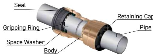
In size 3/4" (22mm), Transair stainless steel pipe uses push to connect technology. Simply push the pipe into the connector until it meets the depth mark on the pipe. The gripping ring will then engage and prevent the pipe from sliding out of the connector.
