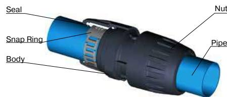
In sizes 2" (50mm) and 2-1/2" (63mm), Transair aluminum pipe uses snap ring technology. Place the snap ring in the two holes at the end of the pipe and slide the nut in-place. Next, hand tighten the nut into the connector body. Lastly, use a pair of spanner wrenches to fully tighten the connector.
