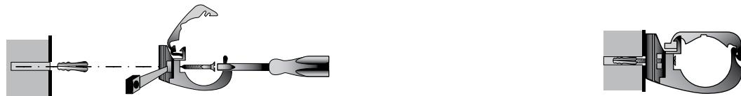
1. Remove the nut at the base of the pipe hanger. Using a screwdriver, insert the screw through the hanger and into the wall. If the hanger does not fall on a stud, use a wall anchor to secure the hanger.
