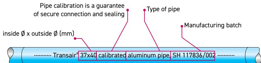
The transported fluid can be instantly identified by the color of the pipe
