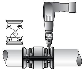
6. Using a drill, fully tighten the clamshell bolts in a cross pattern
