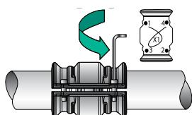
4. Hand-tighten the bolts in a cross pattern with an allen wrench. see chart below for sizes)
