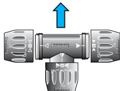
5. Re-tighten the nuts until the empty and solid arrows are aligned with each other.
