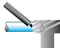
4. Place the marking tool on the end of the pipe, and mark the insertion depth
