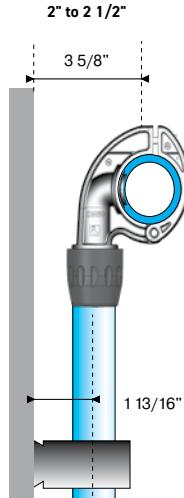
The distance from the center of the pipe to the wall is 1 13/16".
