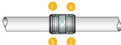
For effective sealing, follow the above diagram for securing the bolts in a cross pattern.
