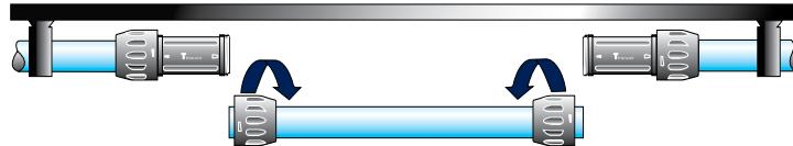
Loosen the nuts on the side of the pipe and slide them away from the connector. Then remove the pipe.
