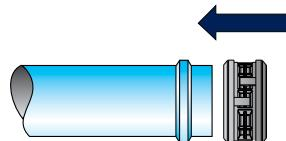
1. Slide the cartridge over the end of the pipe until it meets the lug
