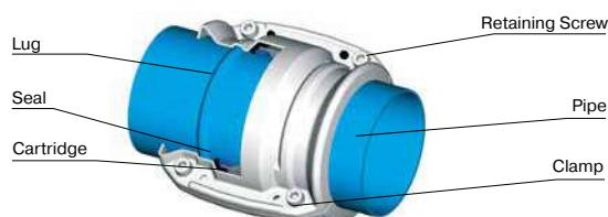
In sizes 3" (76mm), 4" (101mm), and 6" (168mm), Transair aluminum pipe uses clamshell technology. Place the cartridge on the pipe so it meets the lug. Then position the connector so the cartridge is in the middle. Lastly, close the connector and tighten with the provided bolts.
