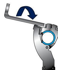
4. Tighten the screw using a 5mm allen wrench
