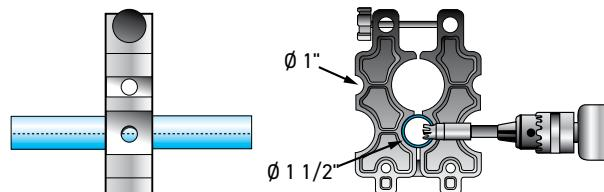
1. Mark the pipe at the desired location, using the dotted line locator marks. These marks will ensure all drop lines off a single piece of pipe will be uniformly aligned. Loosen the retaining bolt on the drilling jig and place it around the pipe. Align your locator mark in-line with the guide hole on the drilling jig. Once the jig is aligned close and tighten the jig. Lastly, place the appropriate drilling tool in your drill and drill the hole.
