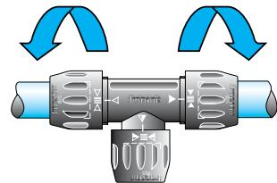
4. Slide the nuts of the tee and position the body of the tee between the 2 pipes such that the solid and empty arrows are facing each other.
