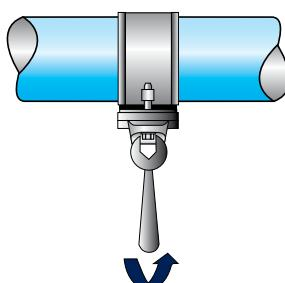
3. Position the plug of the bracket in the hole and tighten the bolts using a crescent wrench
