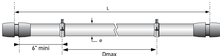
To ensure a stable piping system, Parker Transair suggests the use of at least 2 hangers per pipe. Transair stainless steel pipe should only be mounted using genuine Transair pipe hangers. Additional hangers may be necessary depending on the weight of the media being conveyed. Consult with engineering to determine if additional hangers are necessary.
