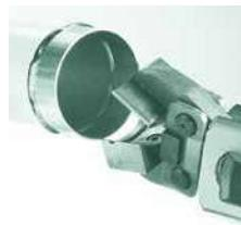
3. Re-open the jaw to remove the pipe. Position the end of the jaw next to the lug mark: this will help to prevent overlapping the lugs.
