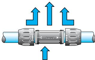
3. Remove the body and nuts of the connector. Re-tighten the nuts onto the body for future use.
