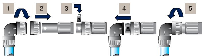
11. Remove the nut on the elbow
