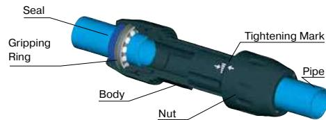
In sizes 1/2" (16,5mm), 1" (25mm), and 1-1/2" (40mm), Transair aluminum pipe uses push to connect technology. Simply push the pipe into the connector until it meets the depth mark on the pipe. The gripping ring will then engage and prevent the pipe from sliding out of the connector.
