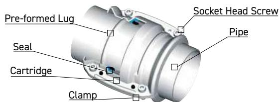
Pipe-to-pipe and stud connectors in Ø76 and Ø101 can be quickly connected to Transair® stainless steel pipe. Position the pipes to be connected within the Transair® cartridge and close/tighten the Transair® clamp.
