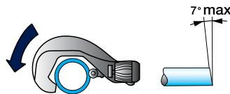
1. Cutting the pipe: Position the blade of the cutter on the pipe, then rotate the pipe cutter around the pipe, gently tightening the blade wheel after each pass.
