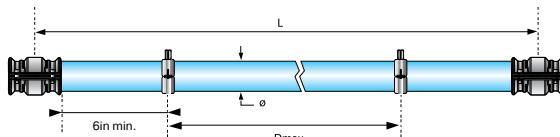
To ensure a stable piping system, Parker Transair suggests the use of at least 2 hangers per pipe. Transair aluminum pipe should only be mounted using genuine Transair pipe hangers.
