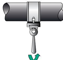
3. Position the plug of the bracket in the hole and tighten the bolts using a crescent wrench.
