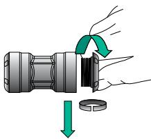
7. Un-thread the end cap and remove the dismounting ring
