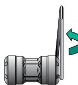
8. Return the end cap and use the dismounting tool to thread the cap back onto the body.
