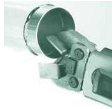
1. Manually open the jaw and insert the stainless steel pipe until the pipe meets the stop in the jaw.
