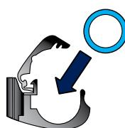
2. Insert the pipe into the pipe hanger
