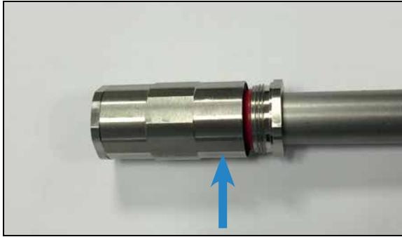
**Disassembly :** 2. Put the red dismounting ring on the pipe and re-screw the nut on the fitting.
