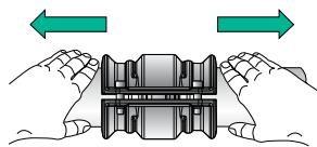
5. Pull the pipes back towards the outside of the clamshell
