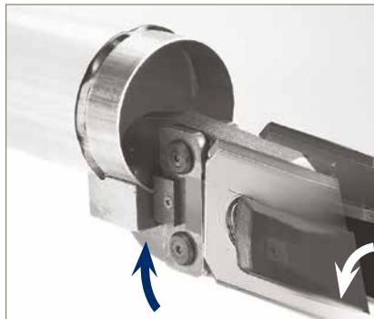
1. Manually open the jaw and insert the aluminum pipe until the pipe meets the stop in the jaw.
