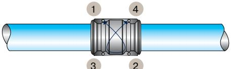
For effective sealing, follow the above diagram for securing the bolts in a cross pattern.
