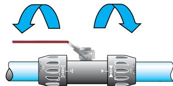
4. Slide the nuts of the valve and position the body of the valve between the 2 pipes so that the empty and solid arrows are facing each other
