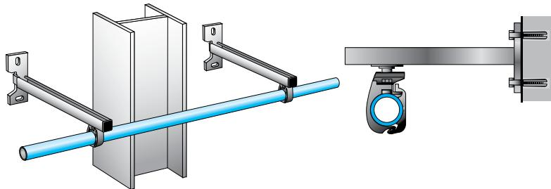
U-channel assemblies are used to offset systems and to bypass obstacles.
