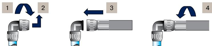
9. Loosen the nut of the elbow
