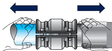
5. Pull the pipe and hose back towards the outside of the clamshell
