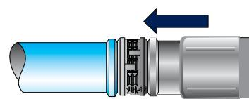
2. Bring the end of the hose to the cartridge and slide the end until the cartridge meets the lug of the hose.
