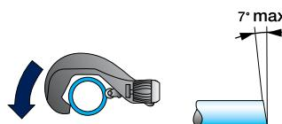
1. Cutting the pipe: Position the blade of the cutter on the pipe, then rotate the pipe cutter around the pipe, gently tightening the blade wheel after each pass.
