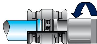
3. Position the clamshell connector over the cartridge/pipe assembly. The cartridge should fall in the middle of the connector
