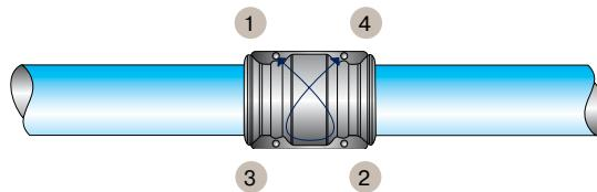
For effective sealing, follow the above diagram for securing the bolts in a cross pattern.
